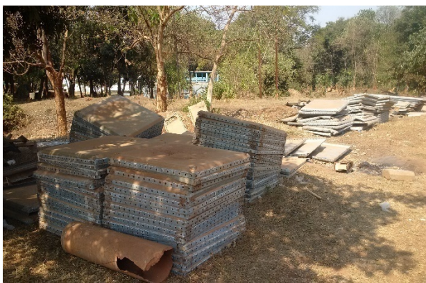
Panels Replaced from Ngwenya tank at LWB Yard
