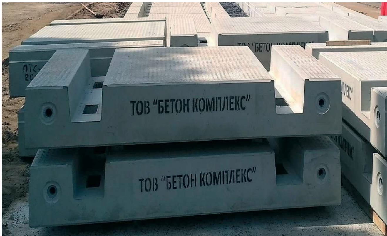
Figure – Construction of block-type tram tracks with 350 mm thick PTS-E reinforced concrete slabs manufactured by PBK Kovalskaya, replaced under the contract for author supervision
