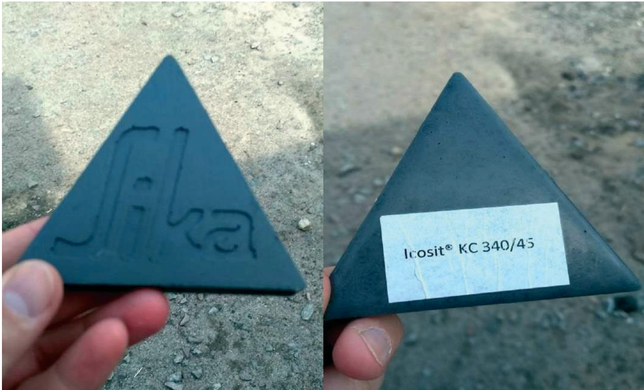
Figure – Sample of Sika Icosit KC polyurethane material used to fix rails in special channels in reinforced concrete slabs
